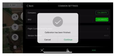
**Notice** if the SharkX appears to shift forward or backward, does uncontrolled circles or does not respond to controls, or flies erratically – land immediately and re-calibrate the compass. If problem still persists, this could be a number of factors including external magnetic or radio interference so contact local distributor/dealer and seek help.
