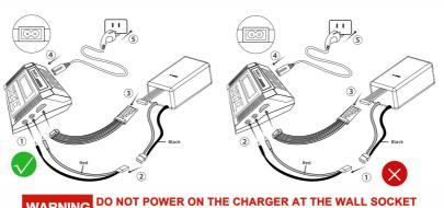
WARNING DO NOT POWER ON THE CHARGER AT THE WALL SOCKET UNTIL THE CABLES ARE ALL CONNECTED PROPERLY
