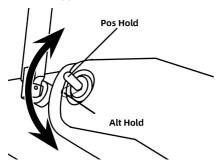
**Notice** always remember to ensure the SharkX is in Position Hold Mode before taking off again
