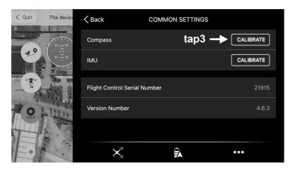
Step 2: Tap 'CALIBRATE' icon and enter the compass calibration interface.
